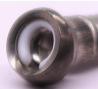
Extragrade Titanium Abutment inclined at 15°. The white Seeger must be positioned with its open side towards the Extragrade bevel.
